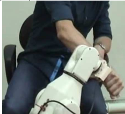
Fig. 9 The training of Kawasaki FS-003N robot by demonstration with using six-component strain sensor.
